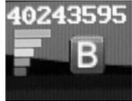
If the 'B' symbol shown is displayed in RED then the handset is out of range of all the base units and cannot be used. Please see section 44 for further details.
