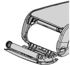
3. Holding the free end of the paper and the terminal, close the printer cover and push firmly until it locks.
